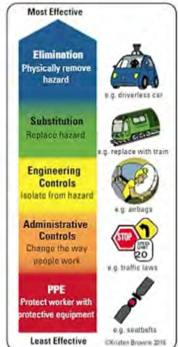
**Figure 18. Hierarchy of controls for reduction of occupational exposures**
